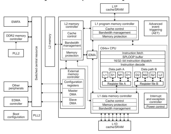
Figure 1. DDR2 Memory Controller Block Diagram
